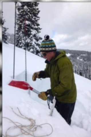
We tested the effect of slope angle on compression tests (CTs) using similar methods as recent ECT work. We collected field data on three separate days with persistent weak layers. Our slopes exhibited gradual changes in steepness, allowing us to sample a variety of slope angles with minimal snow structure changes.
