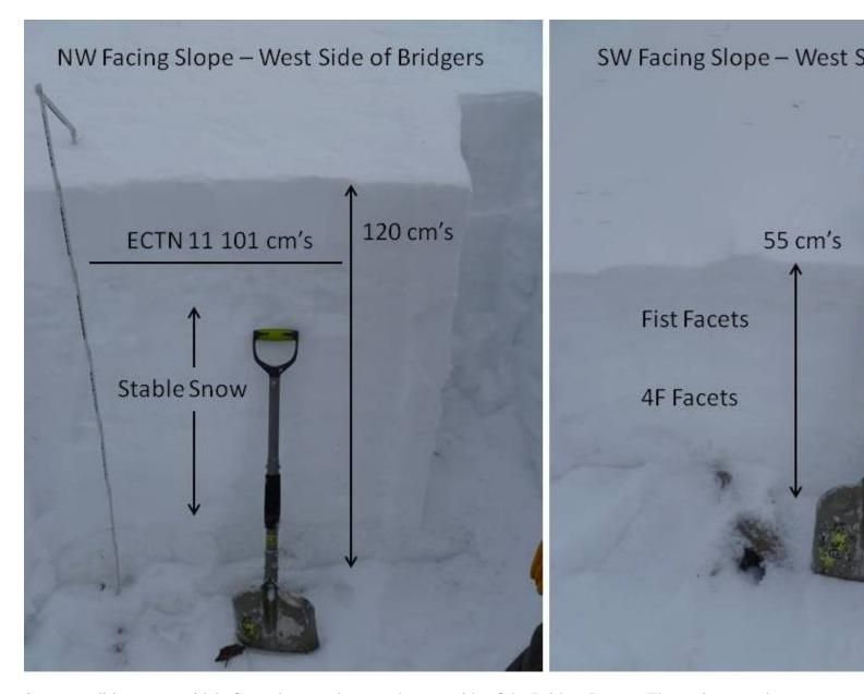
Snow conditions vary widely from slope to slope on the west side of the Bridger Range. These pits were dug only 50 meters apart, but show completely different snowpacks. Photo GNFAC
