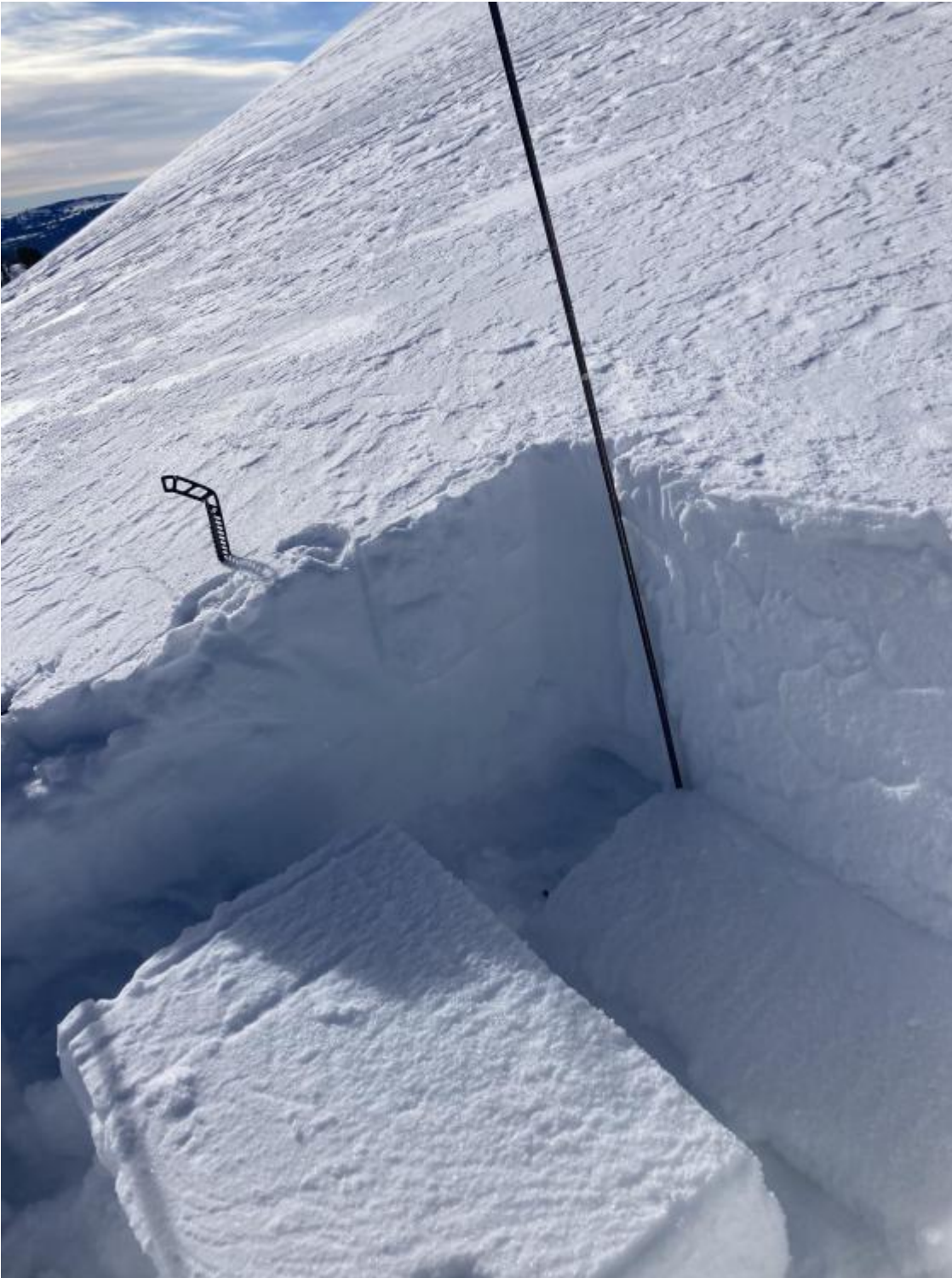
This test broke and propagated with some "extracurricular" hits in an extended column test in Beehive Basin. Photo: N Rustigian
