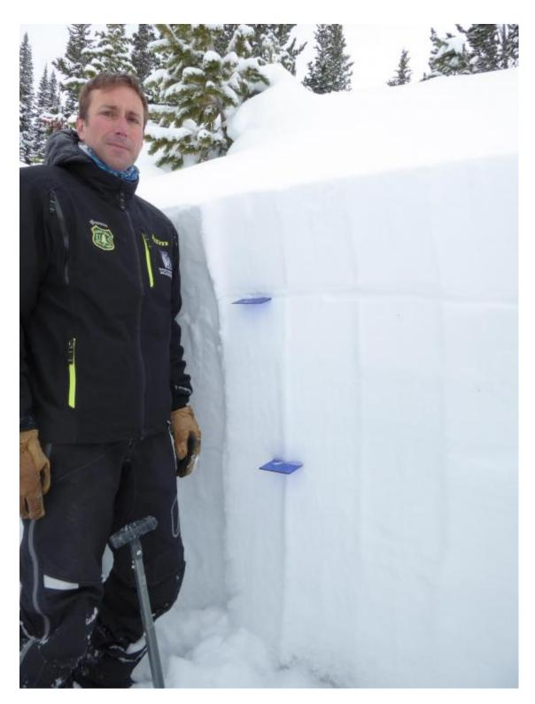
We dug this pit adjacent to a snowmobiler triggered avalanche. It broke on the surface hoar layer which is located at the top blue crystal card. The bottom card denotes the larger grains of facets that formed early in the winter. Photo: GNFAC
