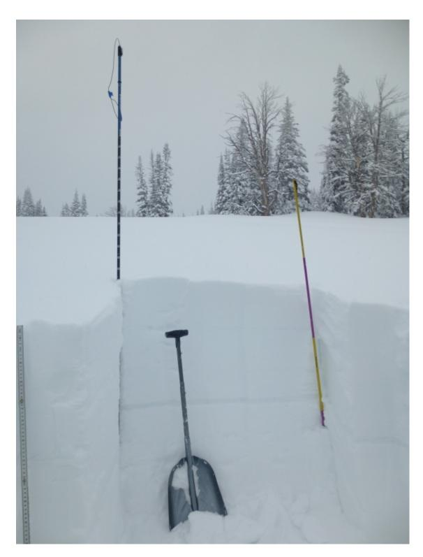
There is 7' of snow on the ground in Bacon Rind (HS 240 cm) and it is stable today. The main concern is the new snow above the ice crust that formed 10 days ago (seen as the stripe behind the shovel) and in two snowpits our stability tests did not propagate. Melting, rain and/or more snow with wind would change the stability, but for now it's good. Photo: GNFAC
